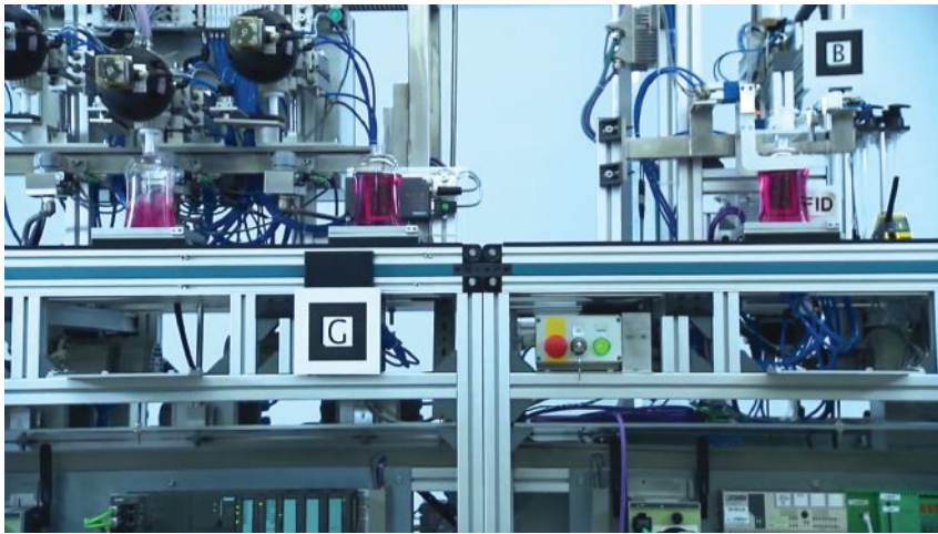
At the German Research Center for Artificial Intelligence, the RFID chip (seen close up on the back of the bottle being filled below) and Siemens hardware are used to communicate instructions to the production equipment for proper processing and quality verification.
