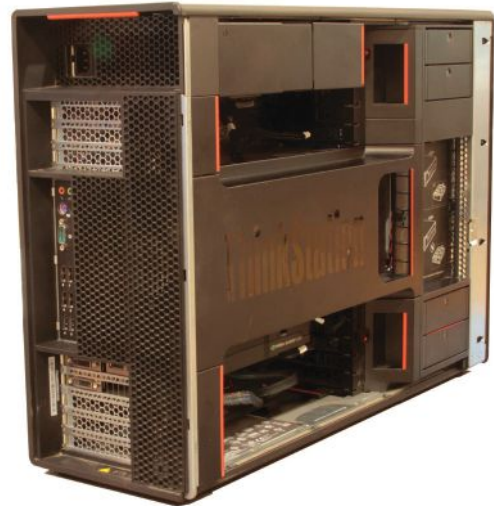
Lenovo's modular design features red touch points, making it easy to remove and replace components.
